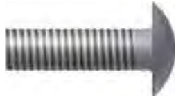
Figure 5-20: 3/8"-16 x 1" Carriage Bolt (2X)
